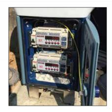
Utilized as an independent or dependent four-channel digital junction box, the SCT-1100 allows for the direct reading and diagnosis of each individual connected load cell or summed as a whole.
