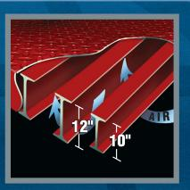
**Competitors'** sealed rib panels can form fatigue cracks in the welds, allowing condensation and rust on the unpainted inside of the supports.
